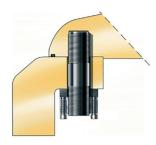
A unique type of bolt is used to install the blades on the hub. The bolts can be tightened using light hand tools from inside the hub.
