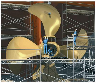
At the shipyard, the ABP offers fast, simple installation compared with a conventional monobloc unit. No match marking is needed
