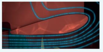
New nozzle profile in a free-running situation. The profile New nozzle profile in towing condition. The shape gives vortex-free flow into and around the nozzle, boosting thrust and thus improving bollard pull.
